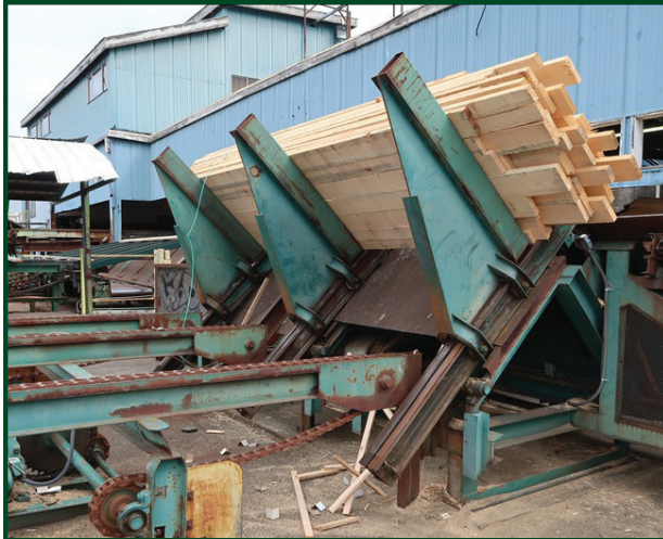
APPROX 12' 3-ARM X 60" MECHANICAL TILT HOIST W/GEARHEAD MOTOR TO BRAKE, APPROX 18' 3-STRAND H78 INFEEED TRANSFER W/HITACHI GEARHEAD MOTOR W/DRIVE
