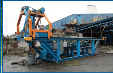
8' VERTICAL BAR TYPE TRAVELING LOG SPLITTER
