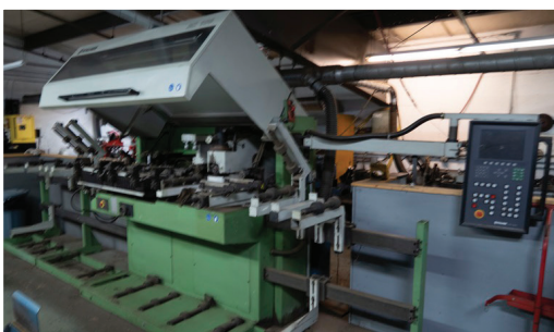
2002 VOLLMER RC100 BANDSAW BENCHING CENTER
