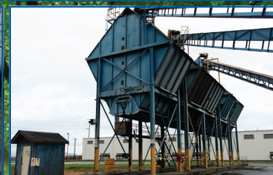
(3) 24-UNIT HYDRAULIC OPERATED CHIP BINS
