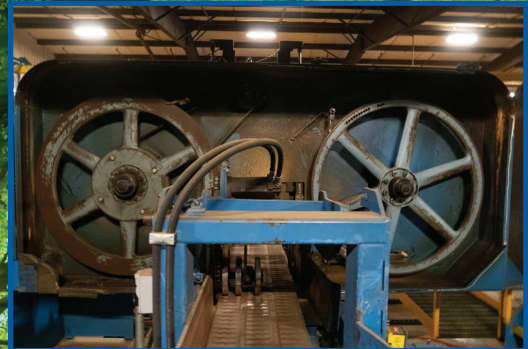
BREWCO LH B1600 SINGLE BAND HORIZONTAL RESAW SYSTEM
