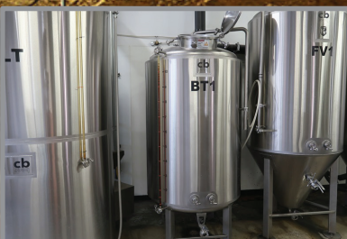
PORTLAND KETTLE WORKS 10 BBL BRIE TANK
