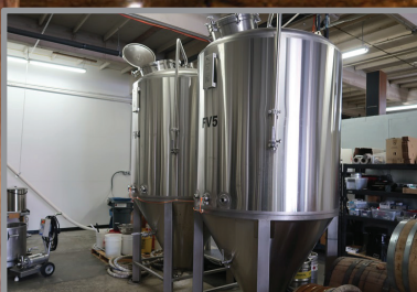
(2) PORTLAND KETTLE WORKS 20 BBL FERMENTATION TANKS
