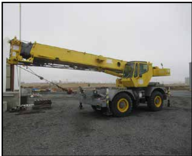
1996 GROVE RT400 22-TON 4X4 ROUGH TERRAIN CRANE, 27'-70' 3-SECTION BOOM, 15' JIB, STANDARD LOAD MOMENT & ANTI 2-BLOCK SYSTEM, CUMMINS 4BT3.9L 6-CYLINDER TURBO DIESEL ENGINE, FULL POWERSHIFT TRANSMISSION, OUTRIGGERS, HOUR METER READS: 7125, S/N: 83430
