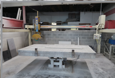
2007 MATRIX BRIDGE SAW W/HYDRAULIC TILT TABLE
