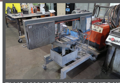
ELLIS 1800 HORIZONTAL BANDSAW
