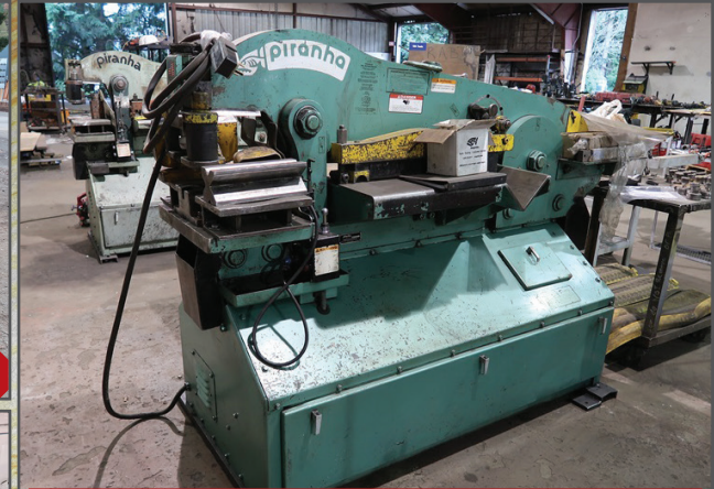
PIRANHA P90 90 TON DUAL STATION IRONWORKER
