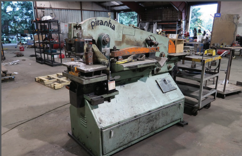
PIRANHA P70 70 TON DUAL STATION IRONWORKER
