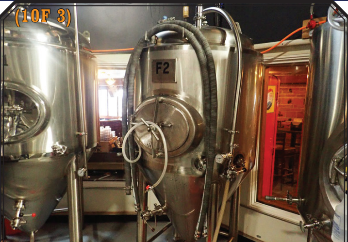
10 BBL S/S JACKETED FERMENTATION TANK
