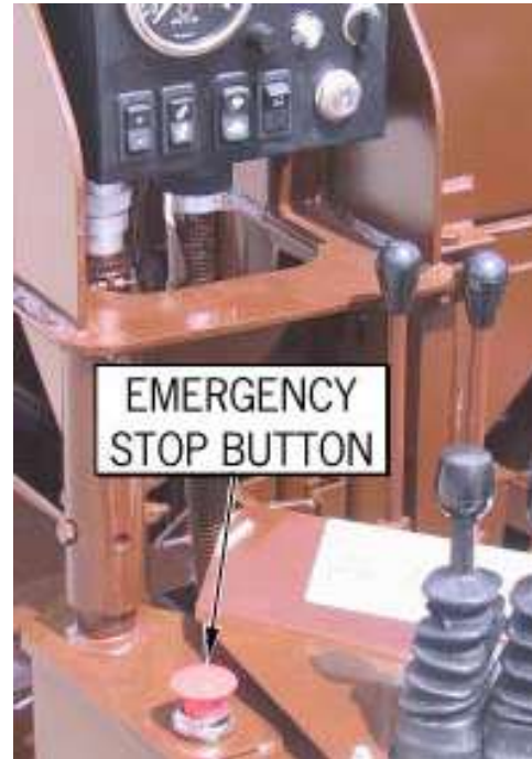
Fig 4-2b Emergency Stop Button - located to left of control levers and under instrument panel.
