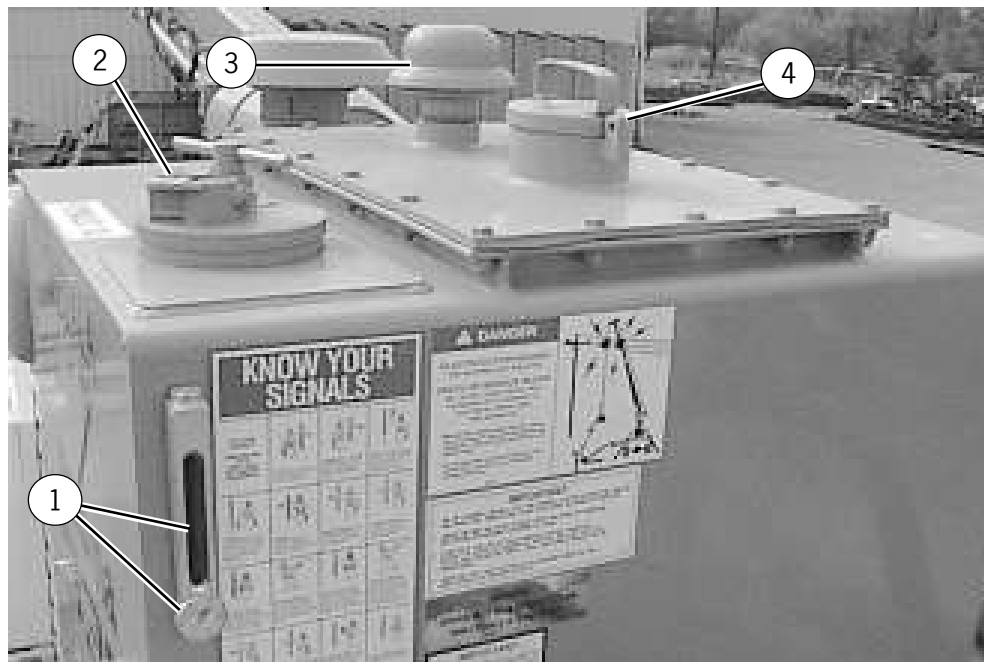
Fig. 5-2 Hydraulic Oil Reservoir
